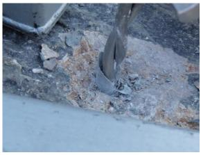
An interesting observation was that the anchors were still holding only a little less than the peak load when half to two thirds of the anchor had been extracted. Whilst no meaningful conclusions can be drawn from the extraction of six bolts it would appear that, because of the styrene, mean failure loads are 10kN higher with the KMR resin.
